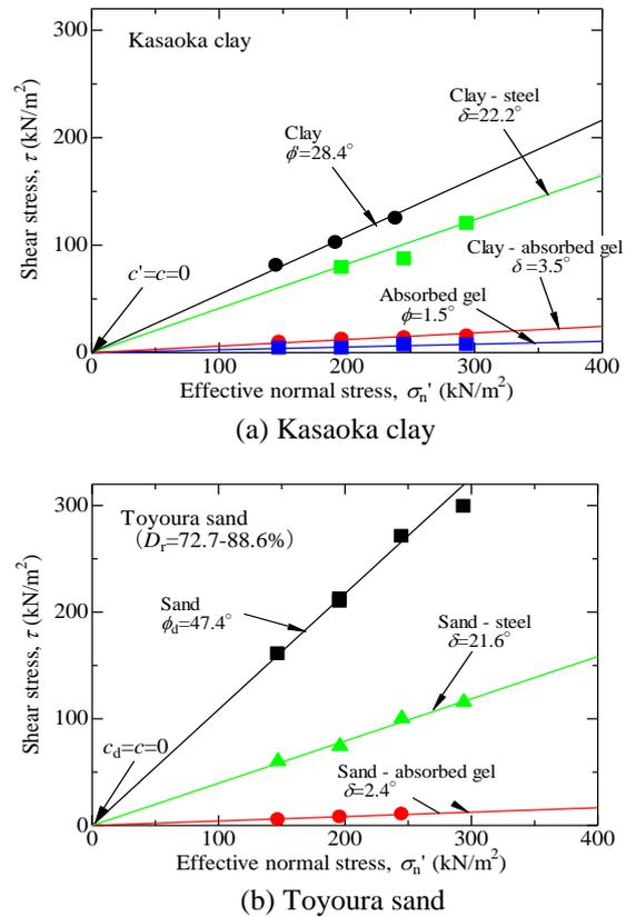
Fig. 12 Internal friction angles and friction angles
