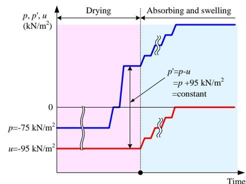
Fig. 4 Test procedure of swelling test
