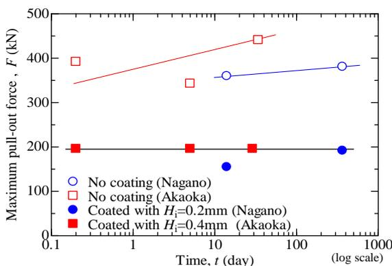
Fig. 13 Maximum pull-out forces in field tests
