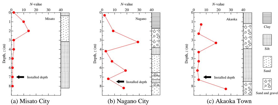
Fig. 7 Ground conditions at test sites in Japan
