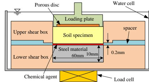
Fig. 6 Cross-section view of specimen and shear box
