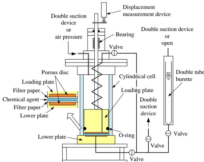
Fig. 3 Column swelling test apparatus
