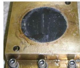
Photo 2. Absorbed gel on steel material after shear test
