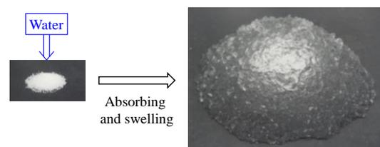
Fig. 2 Absorbing and swelling of superabsorbent polymer
