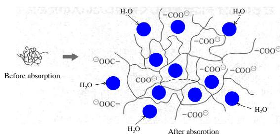
Fig. 1 Absorption mechanism of superabsorbent polymer (Kawakami 2001)
