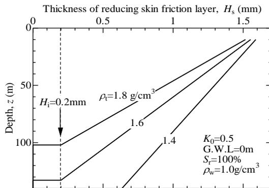
Fig. 10 Trial calculation of the thickness of the layer reducing skin friction
